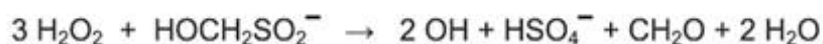
Fig. 3. Scheme of the reaction between sodium formaldehyde sulfoxilate and hydrogen peroxide producing the release of formaldehyde.
