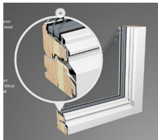
Figure 3: Wooden window with external aluminium cladding. Source: NorDan
