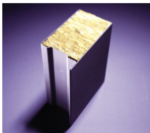
Figure 4: Cross-section of a steel door with a door leaf of 54 mm. The outer layer of thin steel plate encloses mineral wool insulation. Source: Daloc.
